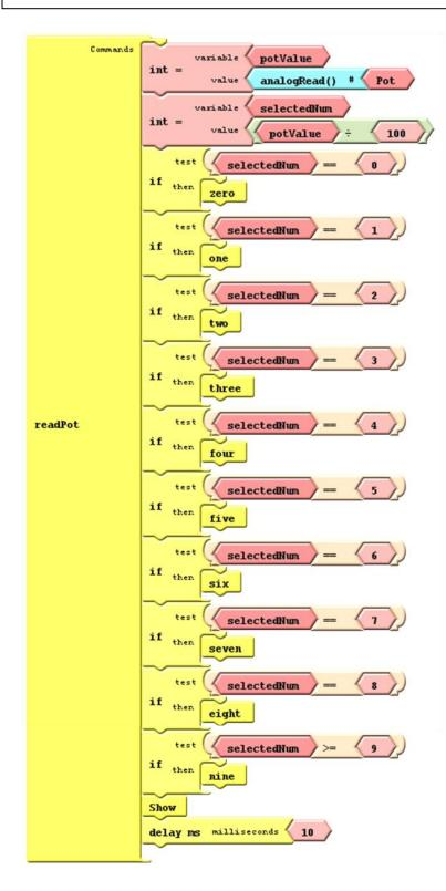
In the "if" statements include a "selectedNum" that reflects the number on the display. This will remain the same when the button is pushed and can be used to insert into digit 1 in the next step.
