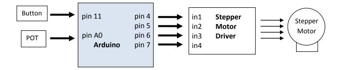
This program turns on two coils at a time. This is called "Full Drive".
