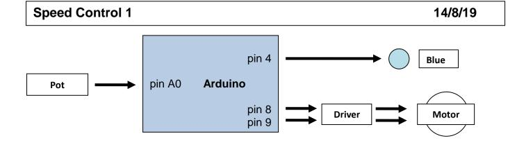
This project will turn on and off the motor/LED forty times a second. (40hz) The motor will be slowed (LED dimmed), depending on how much "ontime" each pulse has compared to the "offtime".
